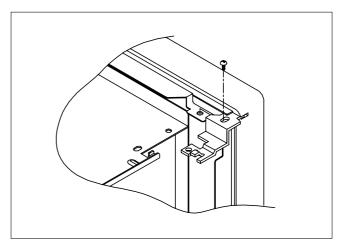
**NOTE**: After replacing the door assembly, perform a check of correct alignment with the hinge and cavity front plate.
